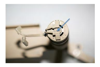
Apply two drops of gun oil or a shot of WD-40 once every couple weeks on the top motor shaft to insure peak performance.
